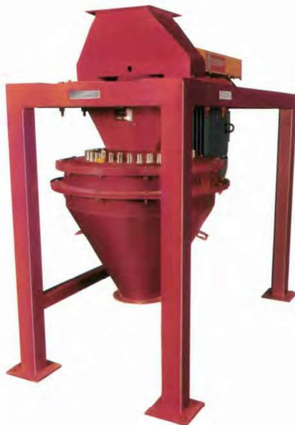
Centrifugal forces move material through alternating stationary and rotating pins.
